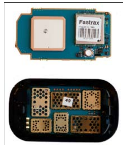
Assisted Bluetooth GPS (BAG) demonstration platform developed by Nokia for R&D purposes only.
